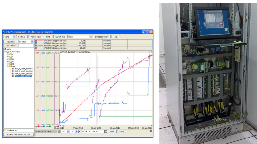
Figure 4.3 Example of processed data trends (VISMON) and a data acquisition cabinet delivered by NGI for placement on an offshore platform
