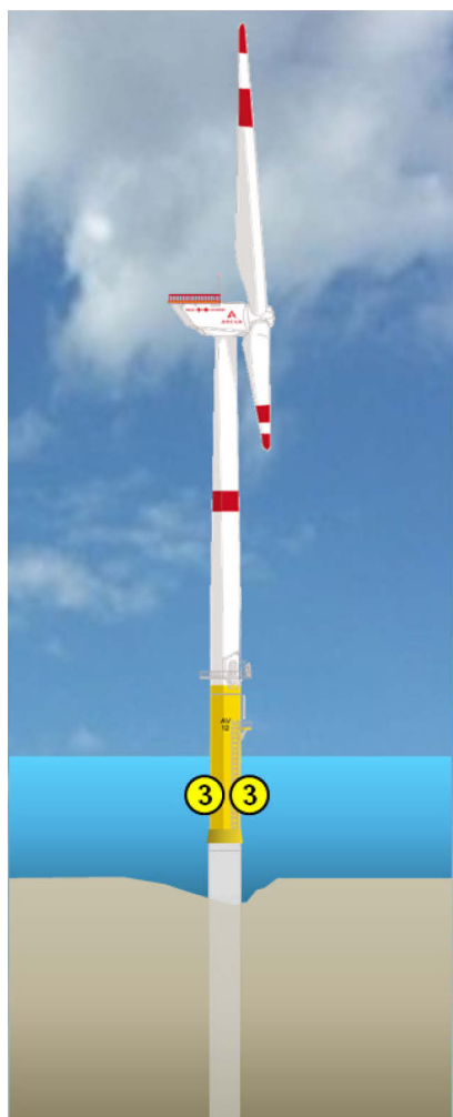
Figure 3.10 Positions of scour sonars on a monopile foundation
