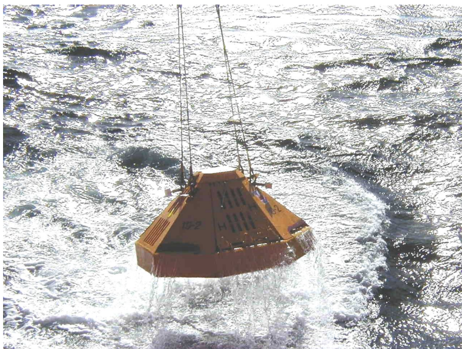
Figure 11.1 NGI seabed monitoring station checked out and deployed into the sea
