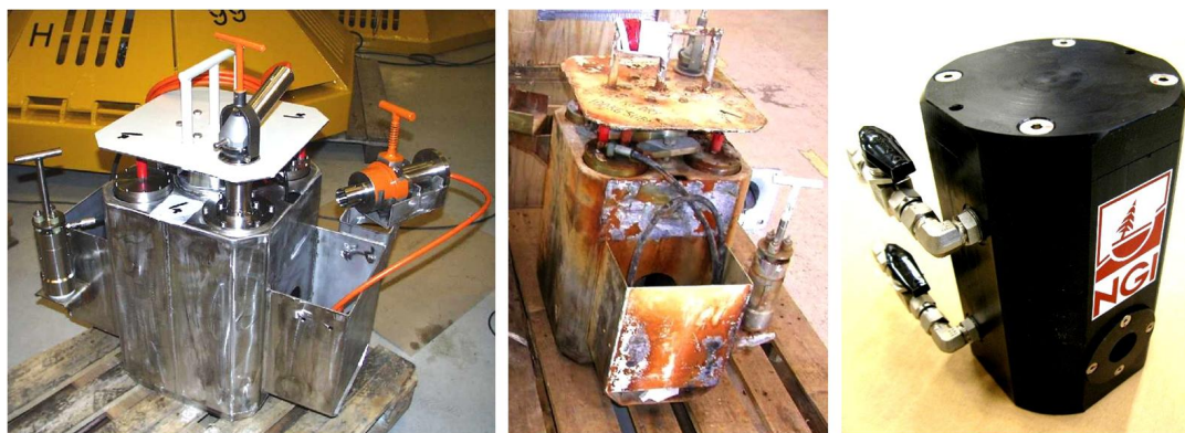
Figure 1.3 “Bright and shiny” instrument unit mainly in stainless steel prior to deployment (left) The same unit heavily corroded after 2 years deployment in seawater (middle). Corrosion “safe” instrument housing made of Delrin with outfitting in stainless (right)
