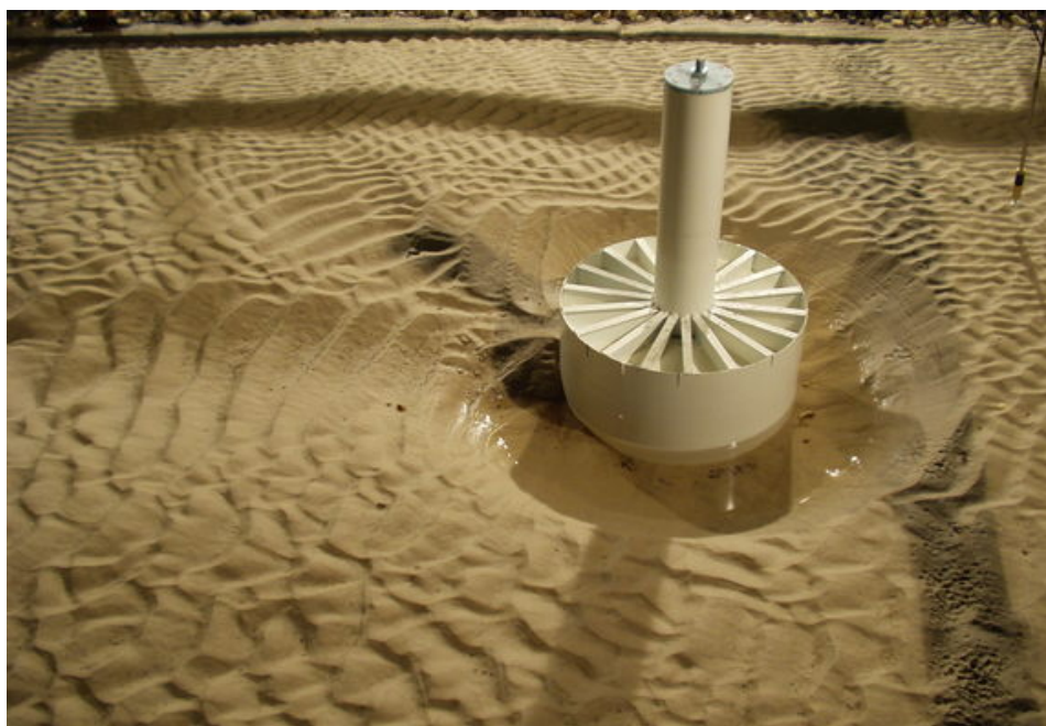
Figure 2.9 Scour pattern after basin testing of a mono caisson foundation (HR Wallingford)
