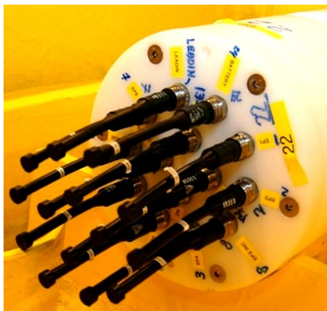
Figure 9.3 Not mated connectors should always be protected by dummy connectors!
