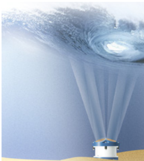
Figure 3.5 ADCP from TeledyneRDI (left) and typical wave and current data (right). Time history showing heights of individual waves (below)
