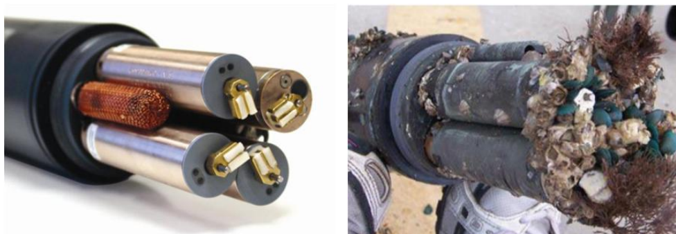
Figure 12.4 Sensor head before installation and with marine growth after some months of operation in tropical waters
