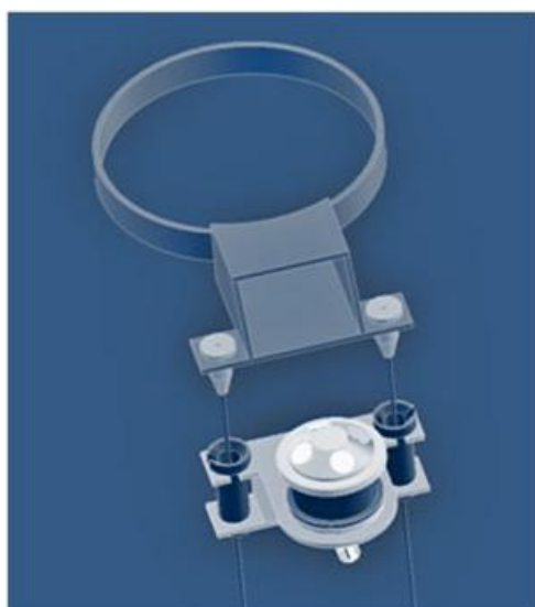
Figure 3.1 Hoisting system for Acoustic Doppler instrument (AWAC) from Abyssus A/S
