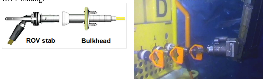
Figure 9.5 Subsea mateable connection with ROV stab on cable end with and panel mounted bulkhead receptacle
