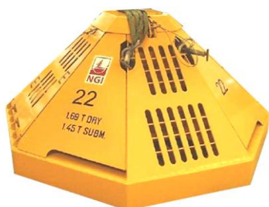
Figure 12.3 NGI's seabed monitoring station with trawling shield and shallow skirts
